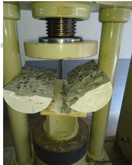
Fig. 3 Split tensile strength testing
