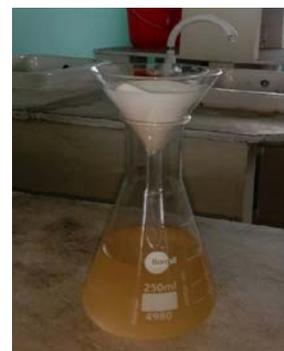
The amount of solids retained in the filter paper is Total suspended solids. The obtained results of Total suspended solids of sample of wastewater is 1008 mg/l, the treated water with Alum is 12 mg/l, the treated water with Ferrous Sulphate is 4 mg/l and the treated water with Poly aluminium Chloride is 0.
