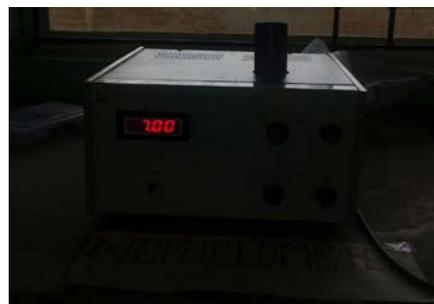
Turbidity is a measure of resistance of water to the passage of light through it. It is due to the presence of suspended mineral matters. The turbidity can be measured using Nephelometer or Turbidity meter. The obtained turbidity of sample of wastewater is 8 NTU, the treated water with Alum is 7.5NTU, the treated water with Ferrous Sulphate is 7 NTU and the treated water with Poly aluminium Chloride is 4.5 NTU.
