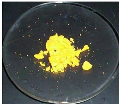
PACl is a relatively new polymeric aluminium coagulant. It is produced under controlled conditions by the partial neutralization of aluminium salts. It shall be in the form of liquid or powder, each of two types: (a) Medium basicity, and (b) High basicity, both grades are effective coagulant for the treatment of low to high turbidity surface raw water for drinking purposes.
