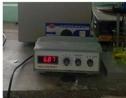
pH refers to the hydrogen ion activity. It is expressed as the negative logarithm of the reciprocal of the hydrogen ion activity in moles per litre. It can be measured by pH meter or using a standard hydrogen electrode and a reference electrode. The obtained pH of sample of wastewater is 6.5, the treated water with Alum is 8.72, the treated water with Ferrous Sulphate is 8.5 and pH of the treated water with Poly aluminium Chloride is 6.87.
