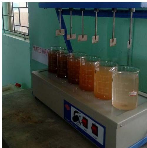
Different doses of coagulant are added to measured volume of samples. The minimum dose of coagulant that produces the lowest residual turbidity is taken as the optimum dosage. From the experiment the Optimum Coagulant Dosage of alum, ferrous sulphate and PACl are 100mg/l, 80mg/l and 40mg/l.
