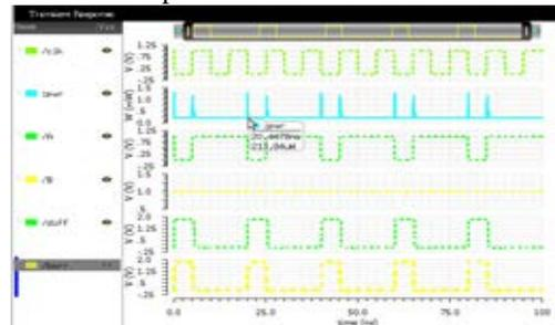
Figure 11: Output waveform of half-subtractor incorporated with AVLS. The power consumption of power gating circuitry is mainly consumed by the sleep transistor.
