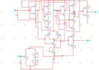
Figure 6: circuit diagram of half sub-tractor AVLG technique
