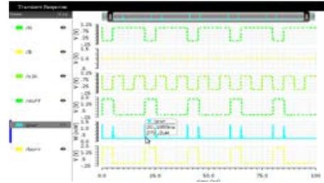
Figure 10: Output waveform of half-subtractor incorporated with AVLG. Here the simulation output shows that the power consumption will be reduced lightly when compared with conventional half-subtractor simulation result. Half-subtractor incorporated with AVLS circuit has a power consumption and propagation delay which is less than the half-subtractor incorporated with AVLG circuit.
