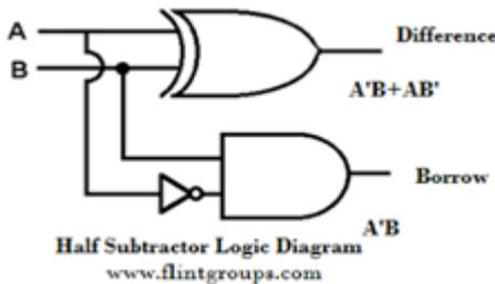
Figure 2: logic diagram of half subtractor
