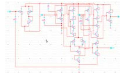
Figure 7: circuit diagram of half subtractor using AVLS technique
