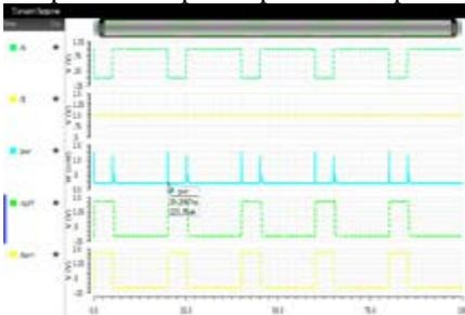
Figure 9: Output waveform of conventional half-subtractor
